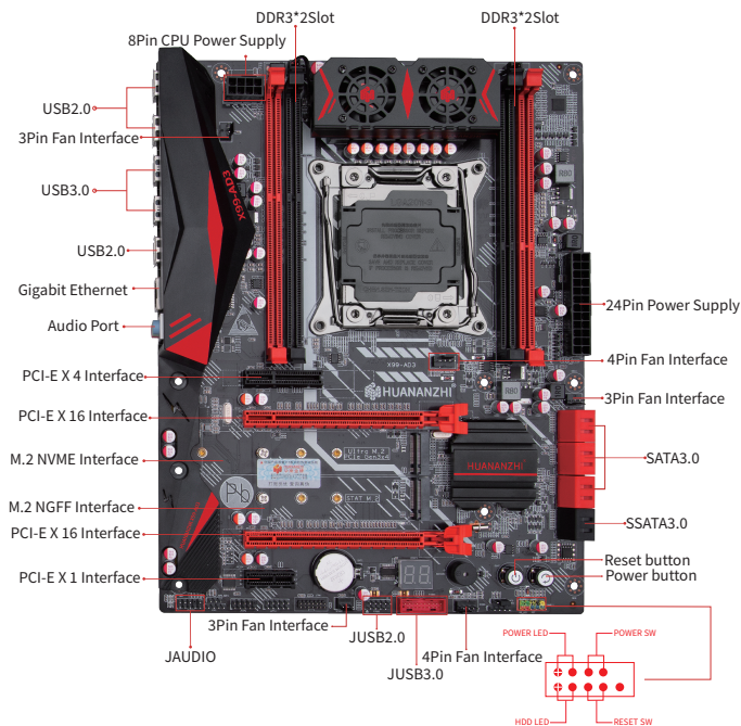
1-1 X99-AD3 V3.0 Motherboard Illustration
